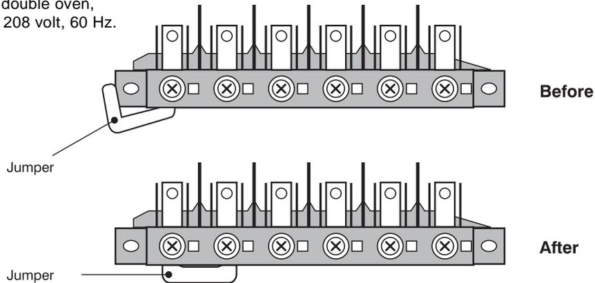
Placing of jumper for lower oven of double oven, for connection to 208 volt, 60 Hz.
