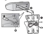
3 Insert the hooks on the wall mounting adaptor into holes (2) and (3) on the base unit.
