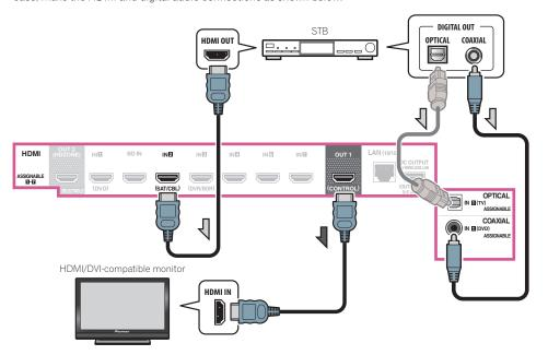
—If you use a digital audio cable or RCA (analog) audio cable, you'll need to tell the receiver which digital input you connected the set-top box to (see <a href="https://linearchy.org/receiver-new-no-page-37">The Input Setup menu</a> on <a href="https://page-37">page-37</a>).
