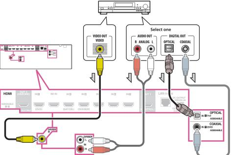
• If your HDD/DVD recorder, BD recorder, etc., is equipped with an HDMI output terminal, we recommend connecting it to the receiver's **HDMI DVR/BDR IN** terminal. When doing so, also connect the receiver and TV by HDMI (see Connecting using HDMI on page 24).
