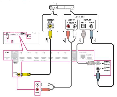
• If your set-top box is equipped with an HDMI output terminal, we recommend connecting it to the receiver's **HDMI SAT/CBL IN** terminal. When doing so, also connect the receiver and TV by HDMI (see Connecting using HDMI on page 24).
