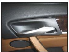
**STEP 2**Carefully pry up on the trim piece around the release handle and remove it from the vehicle.
