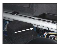
**STEP 28**Slide a U-Nut over the factory hole in the rail as indicated.
