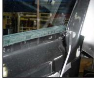
**STEP 8**Unclip the rear of the upper door trim as shown, and remove the panel from the vehicle.
