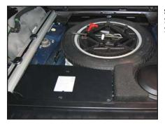
STEP 48 Secure the Battery Cover using the three #8 x 1" Sheet Metal Screws. Reinstall the floor panel.
