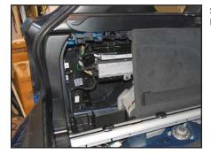
**STEP 30**Remove the access door from the left side panel.
