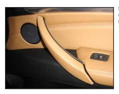
**S T E P 4**Carefully pry off the trim on the pull handle and remove it from the vehicle.
