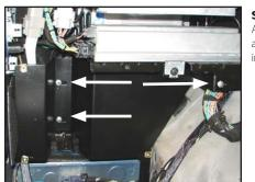
Align the Amplifier Bracket to the factory studs as shown, and secure it to the vehicle using three 5mm Hex Nuts as indicated.
