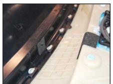
**STEP 10**Cut a second piece of the Foam Tape and apply it to the panel, over the clip as shown.
