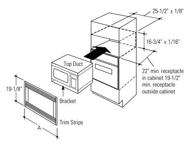
Installation option shown includes: ZE2160 full-size microwave oven built-in with a JX2127SS trim kit above a GE Monogram 27" single wall oven or a JX2130SS trim kit above a GE Monogram 30" single wall oven.
