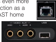
LAN terminal on rear panel (top) and front panel Video Aux terminals with USB port (bottom)
