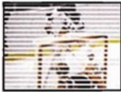
Interlace scanning first scans the odd-numbered lines in 1/60th of a second...
